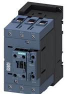
power contactor, AC-3e/AC-3, 95 A, 45 kW / 400 V, 3-pole, 42 V AC, 50/60 Hz, auxiliary contacts: 1 NO + 1 NC, screw terminal, size: S3  $\,$
