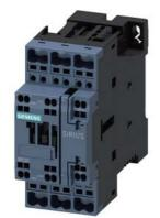
power contactor, AC-3e/AC-3, 9 A, 4 kW / 400 V, 3-pole, 24 V DC, 0.7-1.25\* Us, with plugged-in varistor, auxiliary contacts: 1 NO + 1 NC, spring-loaded terminal, size: S0, suitable for PLC outputs, not expandable with auxiliary switch
