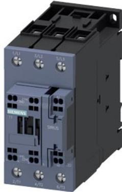
power contactor, AC-3e/AC-3, 65 A, 30 kW / 400 V, 3-pole, 20-33 V AC/DC, 50/60 Hz, with integrated varistor, auxiliary contacts: 1 NO + 1 NC, main circuit: screw terminal, control and auxiliary circuit: spring-loaded terminal, size: S2,
