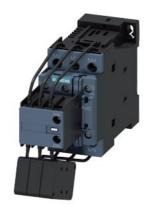
capacitor contactor, AC-6b 25 kVAr, / 400 V, 3-pole, 95-130 V AC/DC, 50/60 Hz, with integrated varistor, auxiliary contacts: 1 NO + 2 NC, screw terminal, size: S0
