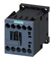
power contactor, AC-3e/AC-3, 12 A, 5.5 kW / 400 V, 3-pole, 220 V DC, auxiliary contacts: 1 NO, screw terminal, size: S00  $\,$
