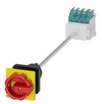
SENTRON, Switch disconnector 3LD, emergency switching-off switch, 4- pole, lu: 16 A, operating power / at AC-23 A 400 V: 7.5 kW, floor mounting with door coupling, rotary operating mechanism, Red / yellow, central mounting 22.5 mm of the handle
