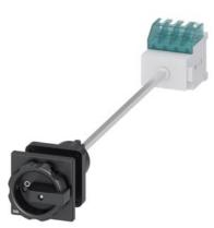
SENTRON, Switch disconnector 3LD, main switch, 3-pole, Iu: 16 A, Operating power / at AC-23 A at 400 V: 7.5 kW, floor mounting with door coupling, rotary operating mechanism, black, central mounting 22.5 mm of the handle
