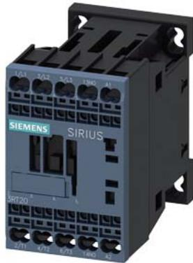
power contactor, AC-3e/AC-3, 16 A, 7.5 kW / 400 V, 3-pole, 110 V AC, 50/60 Hz, auxiliary contacts: 1 NO, spring-loaded terminal, size: S00
