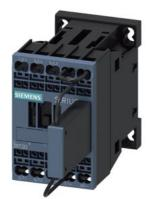
traction contactor, AC-3e/AC-3, 12 A, 5.5 kW / 400 V, 3-pole, 24 V DC, 0.7-1.25\* Us, with integrated suppressor diode, auxiliary contacts: 1 NC, spring-loaded terminal, size: S00, with plugged on series resistor
