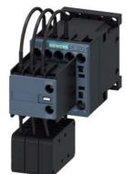
capacitor contactor, AC-6b 12.5 kVAr, / 400 V, 3-pole, 110 V AC, 50 Hz / 120 V, 60 Hz, auxiliary contacts: 1 NO + 1 NC, screw terminal, size: S00
