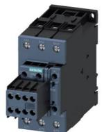
power contactor, AC-3e/AC-3, 65 A, 30 kW / 400 V, 3-pole, 20-33 V AC/DC, 50/60 Hz, with integrated varistor, auxiliary contacts: 2 NO + 2 NC, screw terminal, size: S2, removable auxiliary switch
