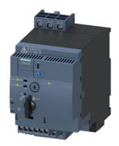
SIRIUS Compact load feeder Reversing starter 690 V 24 V AC/DC 50...60 Hz 0.32...1.25 A IP20 Connection main circuit: Screw terminal Connection control circuit: screw terminal
