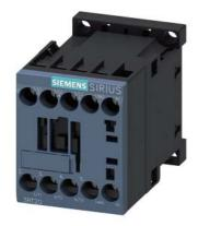
power contactor, AC-3e/AC-3, 9 A, 4 kW / 400 V, 3-pole, 400 V AC, 50 Hz / 400-440 V, 60 Hz, auxiliary contacts: 1 NO, screw terminal, size: S00
