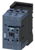
power contactor, AC-3e/AC-3, 95 A, 45 kW / 400 V, 3-pole, 400 V AC, 50 Hz / 400-440 V, 60 Hz, auxiliary contacts: 1 NO + 1 NC, size: S3 removable auxiliary switch
