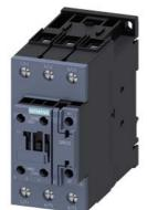
power contactor, AC-3e/AC-3, 80 A, 37 kW / 400 V, 3-pole, 220 V AC, 50/60 Hz, auxiliary contacts: 1 NO + 1 NC, screw terminal, size: S2
