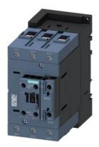
contactor AC-1, 140 A, 690 V / 40 °C, 3-pole, 20-33 V AC/DC, 50/60 Hz, with integrated varistor, auxiliary contacts: 1 NO + 1 NC, main circuit: box terminal, control and auxiliary circuit: screw terminal size: S3
