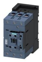
power contactor, AC-3e/AC-3, 80 A, 37 kW / 400 V, 3-pole, 400 V AC, 50 Hz / 400-440 V, 60 Hz, auxiliary contacts: 1 NO + 1 NC, screw terminal, size: S3  $\,$
