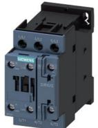
power contactor, AC-3e/AC-3, 9 A, 4 kW / 400 V, 3-pole, 230 V AC, 50/60 Hz, auxiliary contacts: 1 NO + 1 NC, screw terminal, size: S0
