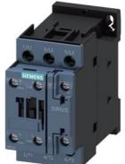
power contactor, AC-3e/AC-3, 12 A, 5.5 kW / 400 V, 3-pole, 110 V AC, 50/60 Hz, auxiliary contacts: 1 NO + 1 NC, screw terminal, size: S0
