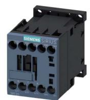
power contactor, AC-3e/AC-3, 12 A, 5.5 kW / 400 V, 3-pole, 24 V DC, 0.7-1.25\* Us, with integrated diode, auxiliary contacts: 1 NC, screw terminal, size: S00, suitable for PLC outputs, not expandable with auxiliary switch
