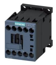
power contactor, AC-3e/AC-3, 12 A, 5.5 kW / 400 V, 3-pole, 42 V AC, 50/60 Hz, auxiliary contacts: 1 NC, screw terminal, size: S00  $\,$
