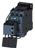
capacitor contactor, AC-6b 20 kVAr, / 400 V, 3-pole, 24 V DC, auxiliary contacts: 1 NO + 2 NC, screw terminal, size: S0
