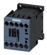
power contactor, AC-3e/AC-3, 12 A, 5.5 kW / 400 V, 3-pole, 24 V DC, 0.7-1.25\* Us, auxiliary contacts: 1 NC, screw terminal, size: S00, suitable for PLC outputs, not expandable with auxiliary switch
