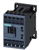
power contactor, AC-3e/AC-3, 7 A, 3 kW / 400 V, 3-pole, 24 V DC, 0.7-1.25\* Us, auxiliary contacts: 1 NO, spring-loaded terminal, size: S00, suitable for PLC outputs, not expandable with auxiliary switch
