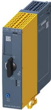
Fail-safe direct-on-line starter High Feature; Electronic switching; Electronic overload protection up to 1.1 kW / 400 V; Adjustment range 0.9 .. 3 A; PROFIenergy; Option: 3DI/LC module
