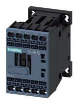
power contactor, AC-3e/AC-3, 7 A, 3 kW / 400 V, 3-pole, 230 V AC, 50/60 Hz, auxiliary contacts: 1 NO, spring-loaded terminal, size: S00, upright mounting position
