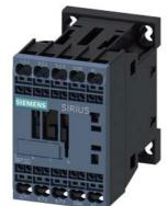
power contactor, AC-3e/AC-3, 9 A, 4 kW / 400 V, 3-pole, 24 V AC, 50/60 Hz, auxiliary contacts: 1 NC, spring-loaded terminal, size: S00
