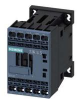
power contactor, AC-3e/AC-3, 7 A, 3 kW / 400 V, 3-pole, 230 V AC, 50/60 Hz, auxiliary contacts: 1 NC, spring-loaded terminal, size: S00, upright mounting position
