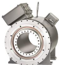
SIMOTICS T Motor de torque completo 1FW3 670rpm, 7.0kW, 100 Nm, 18A, 369V 750rpm, 7.9kW, 100 Nm, 18A, 410V 810rpm, 8.5kW, 100 Nm, 18A, 441V refrigeração a água INCREM. ENCODER SIN/COS 1VPP 2048 S/R (ENCODER IN2048S/R) ENCODER MONTAGEM COAXIAL IMB 14 TERMINAL CAIXA ACIMA: CROSSWISE ESQUERDA Sensor de temperatura KTY OCO EIXO DE PROTEÇÃO IP 54 PADRÃO DE ARMAZENAMENTO
