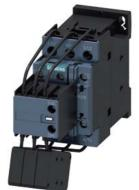
capacitor contactor, AC-6b 25 kVAr, / 400 V, 3-pole, 24 V AC, 50/60 Hz, auxiliary contacts: 1 NO + 2 NC, screw terminal, size: S0
