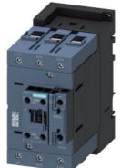
power contactor, AC-3e/AC-3, 110 A, 55 kW / 400 V, 3-pole, 110 V AC, 50/60 Hz, auxiliary contacts: 1 NO + 1 NC, screw terminal, size: S3  $\,$
