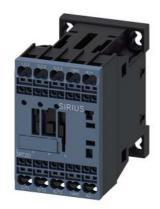
power contactor, AC-3e/AC-3, 7 A, 3 kW / 400 V, 3-pole, 24 V DC, auxiliary contacts: 1 NO, spring-loaded terminal, size: S00, communication-capable
