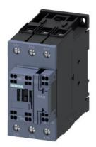
power contactor, AC-3e/AC-3, 65 A, 30 kW / 400 V, 3-pole, 20-33 V AC/DC, 50/60 Hz, with integrated varistor, auxiliary contacts: 1 NO + 1 NC, main circuit: screw terminal, control and auxiliary circuit: spring-loaded terminal, size: S2,
