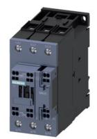
power contactor, AC-3e/AC-3, 65 A, 30 kW / 400 V, 3-pole, 24 V DC, 0.8-1.2\* Us, with integrated varistor, auxiliary contacts: 1 NO + 1 NC, main circuit: screw terminal, control and auxiliary circuit: spring-loaded terminal, size: S2, suitable for PLC outputs
