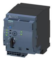
SIRIUS compact starter reversing starter for IO-Link 690 V 24 V DC 1...4 A IP20 connection main circuit: plug-in, without terminals connection control circuit: spring-loaded terminal "phase-out type" alternative 3RK1308 or 3RA8
