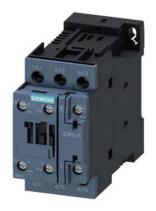
power contactor, AC-3e/AC-3, 12 A, 5.5 kW / 400 V, 3-pole, 24 V DC, 0.7-1.25\* Us, with plugged-in varistor, auxiliary contacts: 1 NO + 1 NC, screw terminal, size: S0, suitable for PLC outputs, not expandable with auxiliary switch
