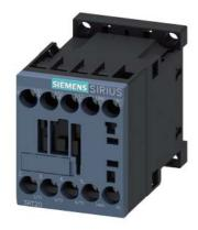
power contactor, AC-3e/AC-3, 7 A, 3 kW / 400 V, 3-pole, 48 V AC, 50/60 Hz, auxiliary contacts: 1 NO, screw terminal, size: S00
