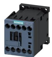
power contactor, AC-3e/AC-3, 12 A, 5.5 kW / 400 V, 3-pole, 400 V AC, 50/60 Hz, auxiliary contacts: 1 NC, screw terminal, size: S00
