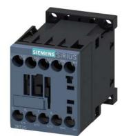
power contactor, AC-3e/AC-3, 12 A, 5.5 kW / 400 V, 3-pole, 24 V DC, 0.7-1.25\* Us, auxiliary contacts: 1 NC, screw terminal, size: S00, suitable for PLC outputs, not expandable with auxiliary switch
