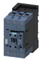
power contactor, AC-3e/AC-3, 80 A, 37 kW / 400 V, 3-pole, 175-280 V AC/DC, 50/60 Hz, with integrated varistor, auxiliary contacts: 1 NO + 1 NC, screw terminal, size: S3
