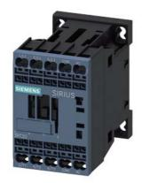
power contactor, AC-3e/AC-3, 9 A, 4 kW / 400 V, 3-pole, 230 V AC, 50/60 Hz, auxiliary contacts: 1 NC, spring-loaded terminal, size: S00  $\,$
