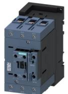
power contactor, AC-3e/AC-3, 95 A, 45 kW / 400 V, 3-pole, 24 V AC, 50/60 Hz, auxiliary contacts: 1 NO + 1 NC, screw terminal, size: S3  $\,$
