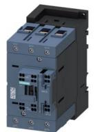
power contactor, AC-3e/AC-3, 80 A, 37 kW / 400 V, 3-pole, 110 V AC, 50/60 Hz, auxiliary contacts: 1 NO + 1 NC, main circuit: screw terminal, control and auxiliary circuit: spring-loaded terminal, size: S3
