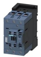
power contactor, AC-3e/AC-3, 80 A, 37 kW / 400 V, 3-pole, 24 V DC, 0.8-1.2\* Us, with integrated varistor, auxiliary contacts: 1 NO + 1 NC, integrated varistor, main circuit: screw terminal, control and auxiliary circuit: spring-loaded terminal, size: S3, suitable for PLC outputs
