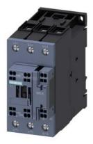
power contactor, AC-3e/AC-3, 80 A, 37 kW / 400 V, 3-pole, 230 V AC, 50/60 Hz, auxiliary contacts: 1 NO + 1 NC, main circuit: screw terminal, control and auxiliary circuit: spring-loaded terminal, size: S2
