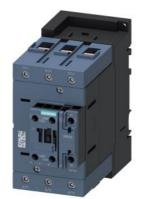
power contactor, AC-3e/AC-3, 80 A, 37 kW / 400 V, 3-pole, 83-155 V AC/DC, 50/60 Hz, with integrated varistor, auxiliary contacts: 1 NO + 1 NC, screw terminal, size: S3
