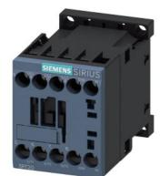
power contactor, AC-3e/AC-3, 9 A, 4 kW / 400 V, 3-pole, 110 V AC, 50/60 Hz, auxiliary contacts: 1 NC, screw terminal, size: S00
