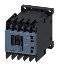
power contactor, AC-3e/AC-3, 7 A, 3 kW / 400 V, 3-pole, 200 V AC, 50 Hz / 200-220 V, 60 Hz, auxiliary contacts: 1 NC, ring cable lug connection, size: S00
