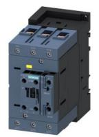
power contactor, AC-3e/AC-3, 95 A, 45 kW / 400 V, 3-pole, 83-150 V AC/DC, 50/60 Hz, with integrated varistor, auxiliary contacts: 1 NC, screw terminal, size: S3, F-PLC-IN
