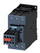
power contactor, AC-3e/AC-3, 80 A, 37 kW / 400 V, 3-pole, 24 V DC, 0.8-1.2\* Us, with integrated varistor, auxiliary contacts: 2 NO + 2 NC, screw terminal, size: S2, suitable for PLC outputs, captive auxiliary switch
